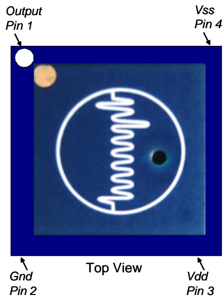
Fig. 4 Pin Assignment for the PS25405B – Top View
