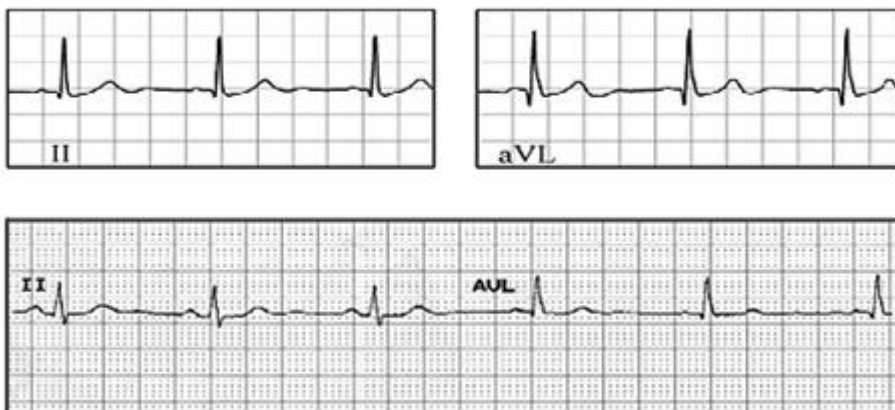
Fig. 8 Comparison of two vectors from a pair of EPIC sensors (top) and two conventional Ag/AgCl electrodes (bottom)
