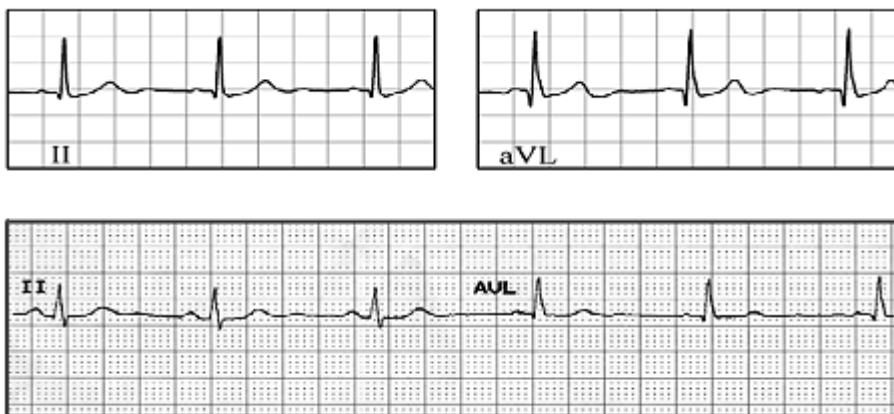
Fig. 8 Comparison of two vectors from a pair of EPIC sensors (top) and two conventional Ag/AgCl electrodes (bottom)
